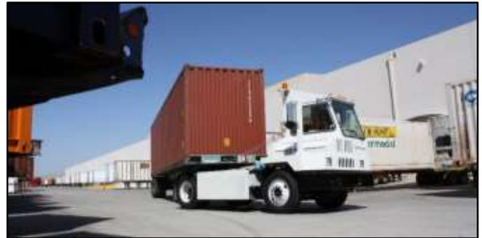
*The Kalmar tractor at IKEA's Tejon Distribution Center features an electric propulsion technology developed by TransPower. A one-year demonstration project, funded in part by the Valley Air District and EPA, showed significant reductions in pollution and fuel savings. (Bottom Photo: TransPower)*
